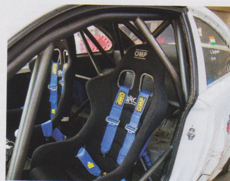
Clockwise from above: Hydraulic handbrake mounted high for ease of operation; it doesn't lock like on road cars. Tyres are chewed up at an alarming rate - these are from the BMW after two flat-out laps. Full roll-cage provides rigidity to the chassis along with safety
