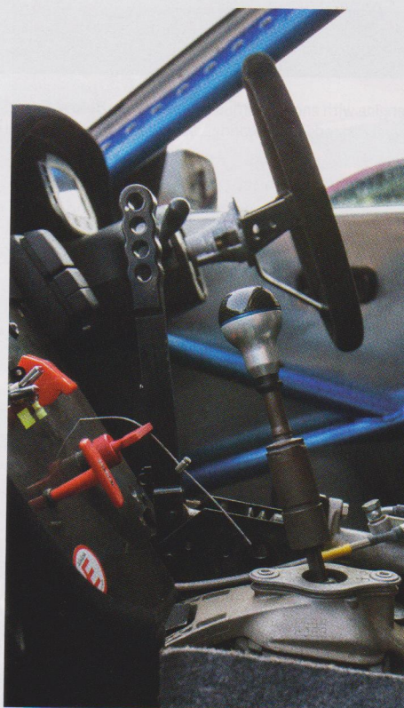
Clockwise from above: Hydraulic handbrake mounted high for ease of operation; it doesn't lock like on road cars. Tyres are chewed up at an alarming rate - these are from the BMW after two flat-out laps. Full roll-cage provides rigidity to the chassis along with safety
