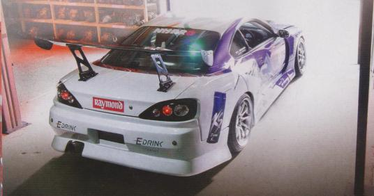
are all there on this S15, from the heavily skirted BN Sports body kit to the vented bonnet (also lifted at the rear for extra cooling) and high-level rear GT wing. Eagle-eyed readers may have spotted that the red and purple colours are shared between the two cars, though the sides are reversed. It is a stimulating scheme inspired by the Kama Sutra energy drink produced by one of Mr Singhania's companies, red being the mixed berry flavour and purple the mixed fruit
