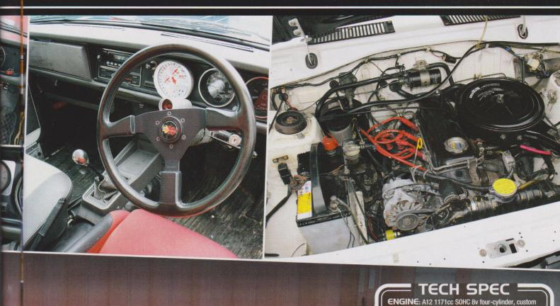
ENGINE: A12 1171cc SOHC 8v four-cylinder, custom motorbike-style exhaust back box. Standard four-speed gearbox
